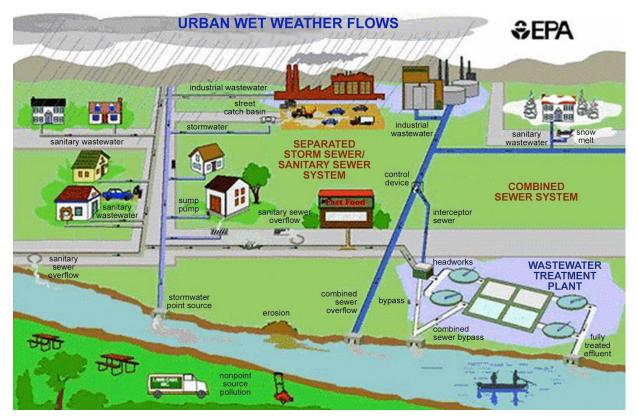
One system is called a **Separated Storm Sewer/Sanitary Sewer System** (see the left side of the EPA graphic). In this system, there are two sets of pipes. One set carries stormwater and nonpoint source pollution from the storm drains and releases it directly into the nearest river or stream without treatment. The other set of pipes carries residential and industrial wastewater to the Wastewater Treatment Plant before it is released into the river.
